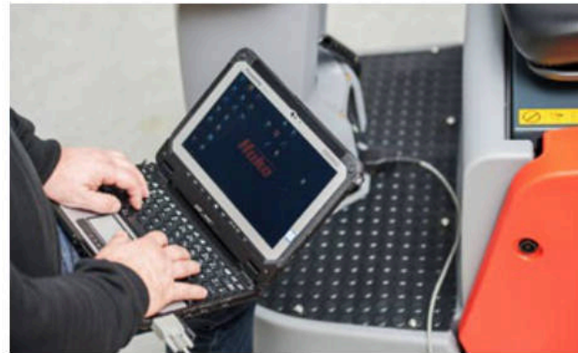
Easy access to the diagnosis interface for maintenance purposes and to modify machine settings.
