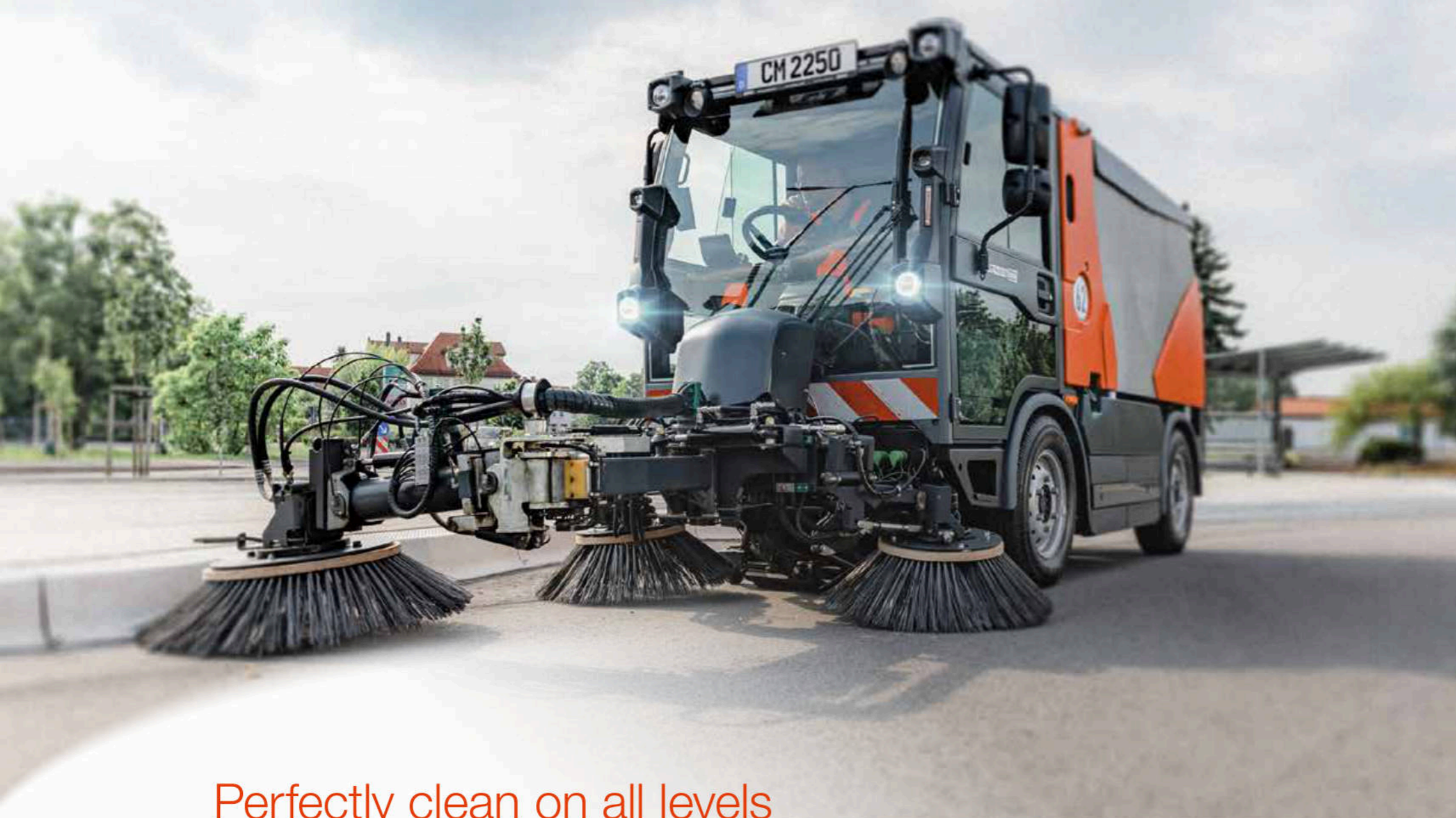
For low-dust sweeping: effective dust control through individually adjustable fresh water nozzles on all disc brushes.
