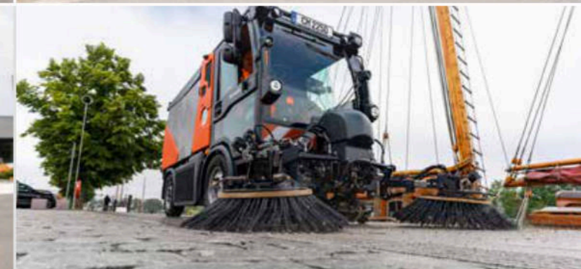
For reliable and safe results: the roller-guided suction duct with rubber sealing strips increases the dirt pick-up capacity – and at the same time reduces collision damage and wear. In addition, the optional suction duct camera provides information about possible material accumulations.
